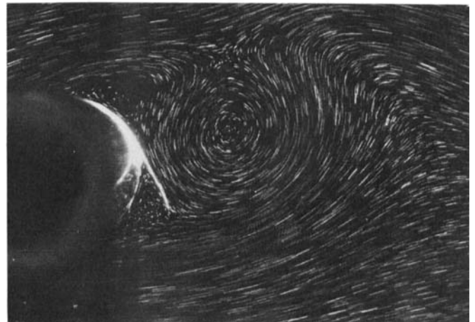
FIGURE 3. Comparison of calculated and experimental instantaneous streamlines for R = 200 ; \alpha = \frac{1}{2} : (a) \tau = 3.0 ; (b) 6.0 ; (c) 9.0 .
